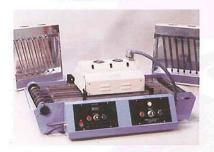
For some potential users of Infra-Red heating, drying or curing systems it is desirable to determine the most appropriate wavelength of emitter before embarking on the purchase of a full -scale system. The Industrial Process Simulator is designed to provide just this facility.
