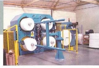
◀This "JUMBO" spooling system is modular in design, using 2 station spooling modules. The Unwind section takes "PRE-SLIT" rolls and can support up to 10 spooling stations. The maximum spool size for this machine is 1200mm diameter x 1000 mm. The maximum speed is 500mpm.
