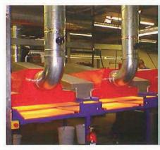
These pictures show good examples for a pre-heat system of infrared being used prior to entry of a stenter drying system. Typically up to 30% of the energy used is to heat up excessive moisture prior to drying.
