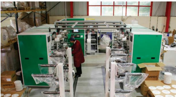
These are our most versatile machines which can process a wide range of materials, both adhesive or non adhesive. These machines dominate the UK Contract Spooling sector. They are modular in design and can be expanded after initial installation. The Unwind section incorporates Guiding and Slitting. Rotary Shear; Rotary Crush; and Razor Slitting cassettes are standard within this model.
