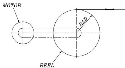
$$\begin{aligned} \text{MOTOR TORQUE} &= \text{TENSION} \times \text{REEL RAD.} \\ \therefore \text{TENSION} &= \frac{\text{MOTOR TORQUE}}{\text{REEL RADIUS}} \end{aligned}$$
