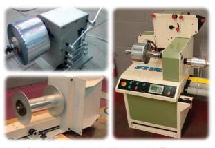
De-spooling units for Holographic Tapes. De-spool/Re-spool salvage units. Traversing slit-edge waste rewind units.
