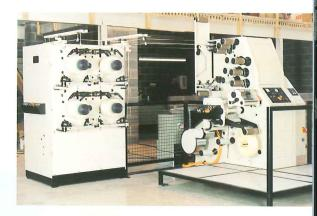
used are optimised to ensure that no edge damage occurs to the material during the winding process, otherwise the next process using the spooled product will suffer.
