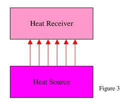
With conductive or convective heat transfer, doubling the source temperature approximately doubles the heat transferred. With radiant heat transfer, doubling the temperature of the source, increases the radiant energy density by a factor of 16.
