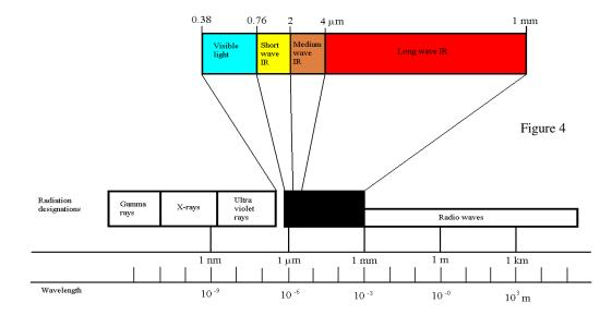
Infra Red is produced as a continuous band of wavelengths in the range of 0.8 microns to 1mm. As temperature is increased the intensity of Infra Red radiant energy increases considerably (proportional to absolute temperature to the power 4, that is  $T^4$ , so if the absolute temperature of an Infra Red emitter is doubled, it will give out 16 times as much Infra Red per unit area of surface – The Stefan-Boltzmann Law).
