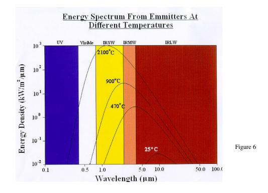
The above data relates to perfect radiators (black bodies). In practice Infra Red emitters have an emissivity of less than 1 so are not perfect emitters, therefore their radiant emission will be lower than that indicated.
