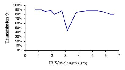
Infra Red Absorption Of Non Pigmented Polyethylene
